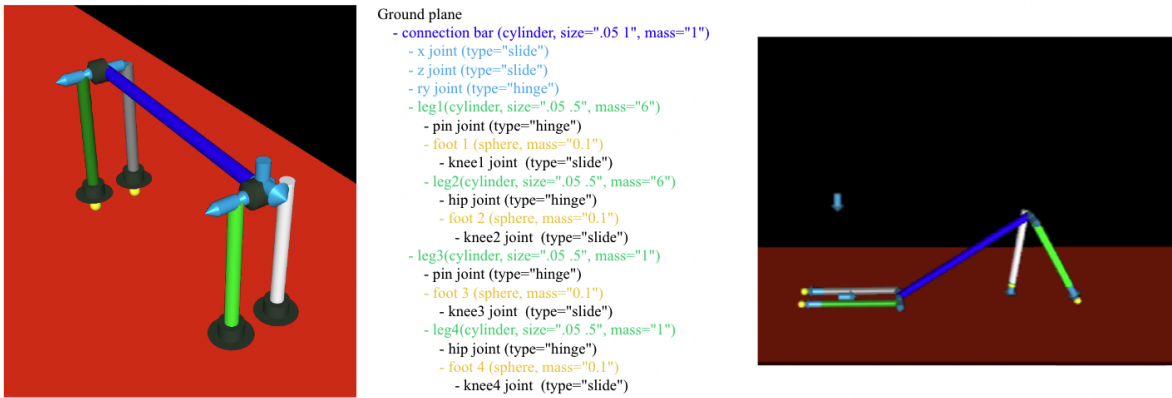
Figure 9: The hierarchical representation of our model and the simulation result of driven by front legs only.
